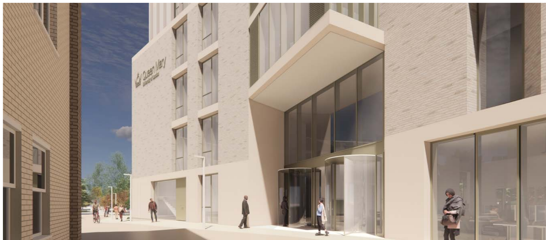
Double height entrance with projecting bay above and precast concrete base surrounding
