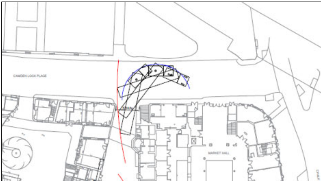
Figure 23 Middle Yard swept path analysis – containers reversed in
