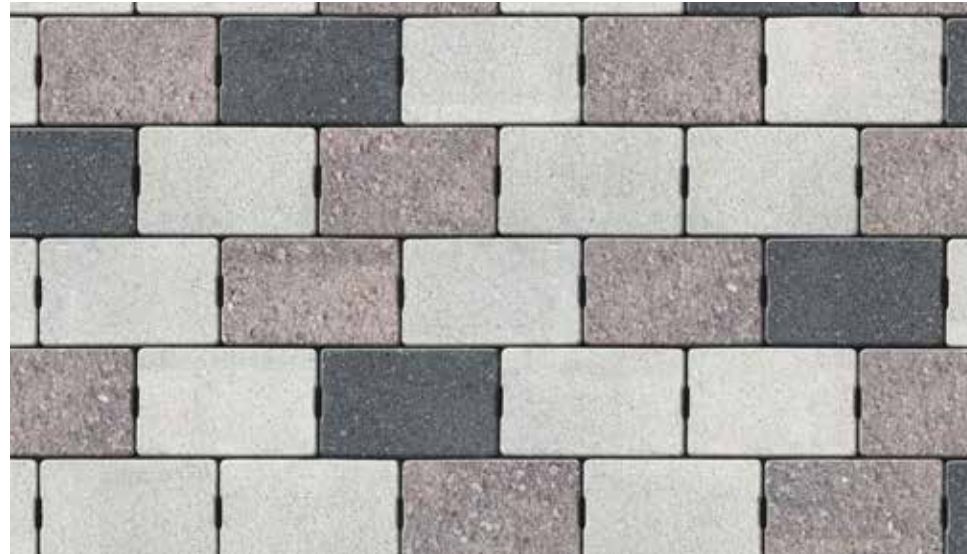
Pedestrian crossovers – Concrete block paver Colour: Mixed blend (3 no.) Mixed sizes: 160 x 120, 160 x 160, 160 x 240mm (60mm thick, except 80mm for raised table/ carriageway zones and to cover 1000mm zone offset from kerblines for vehicular overrun)
