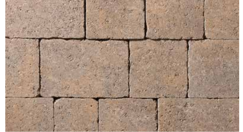
Footway – Concrete block paver Colour: Warmer, monocolour Mixed sizes: 160 x 120, 160 x 160, 160 x 240mm (60mm thick, except 80mm to cover 1000mm zone offset from kerb line for vehicular overrun)
