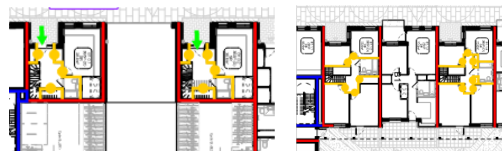
Figure 2: Example Block B1 with 30/30/30 fire-resisting protected hallway
