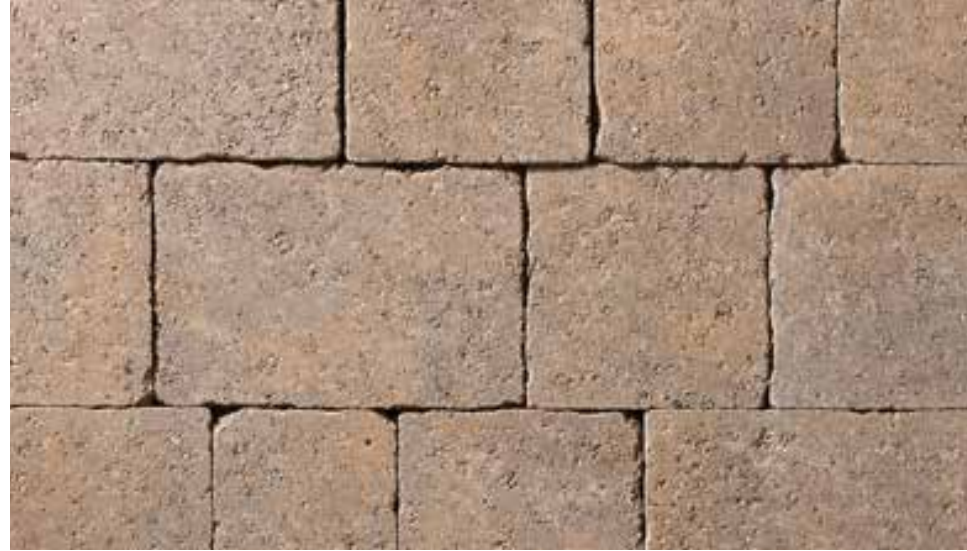
Concrete block paver to Mews footway Colour: Natural, monocolour Mixed sizes: 160 x 120, 160 x 160, 160 x 240mm (60mm thick) *To be laid to permeable build-up as part of SUDs strategy
