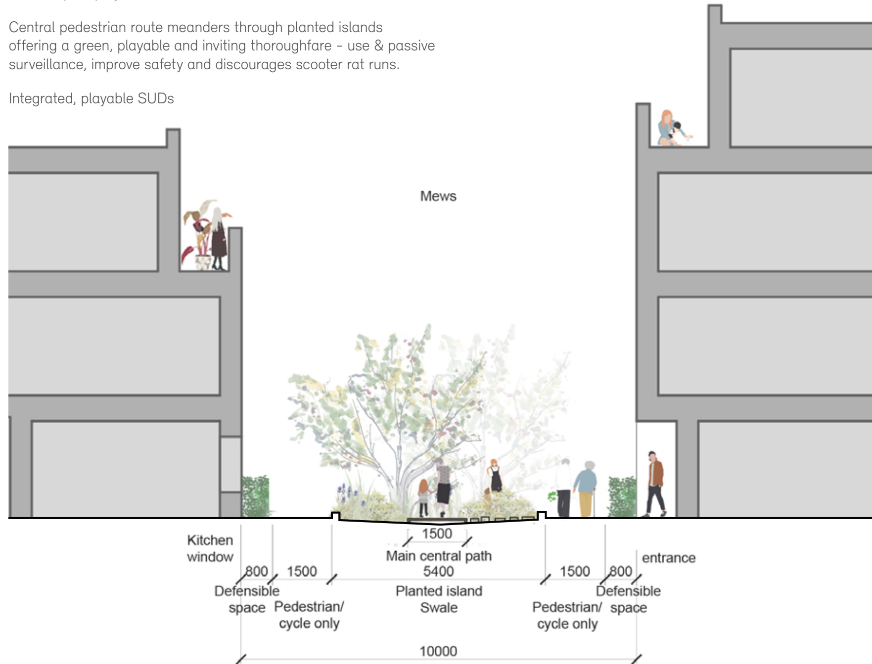
Section through Blocks B4 & B5
