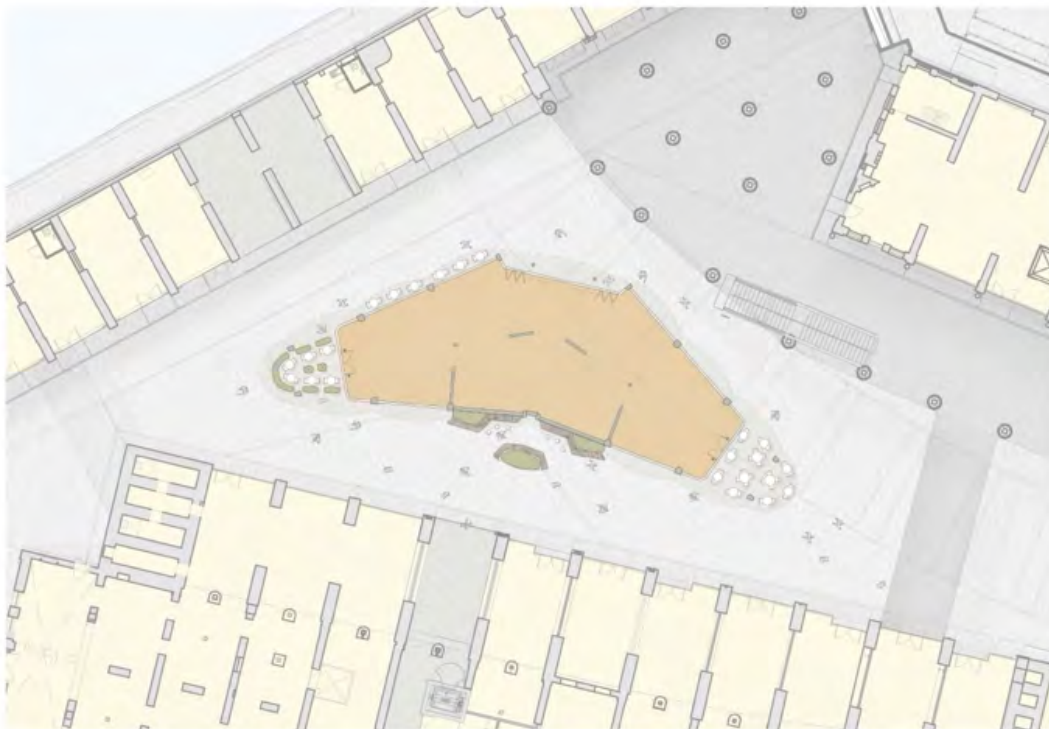
Fig 33: The yard level plan of the proposed pavilion, relates to the grid lines of the surrounding viaduct structures and is defined by their frontages whilst also subtly reflecting the historical fan-like nature of the viaducts in its triangular form.
