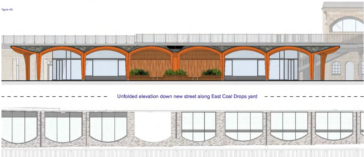
Figs 35: The east elevation of the pavilion reflects the Eastern Viaduct segmental arcading immediately opposite utilising a much lighter timber structure in a contemporary sculptural manner
