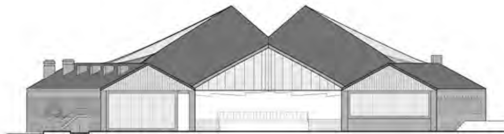
Figs 22 & 23: South (top) and North (bottom) elevations of the Coal Drops Yard development demonstrates the splayed nature of the relationship between the coal drop buildings and the very different nature of the north and south yard spaces that result.
