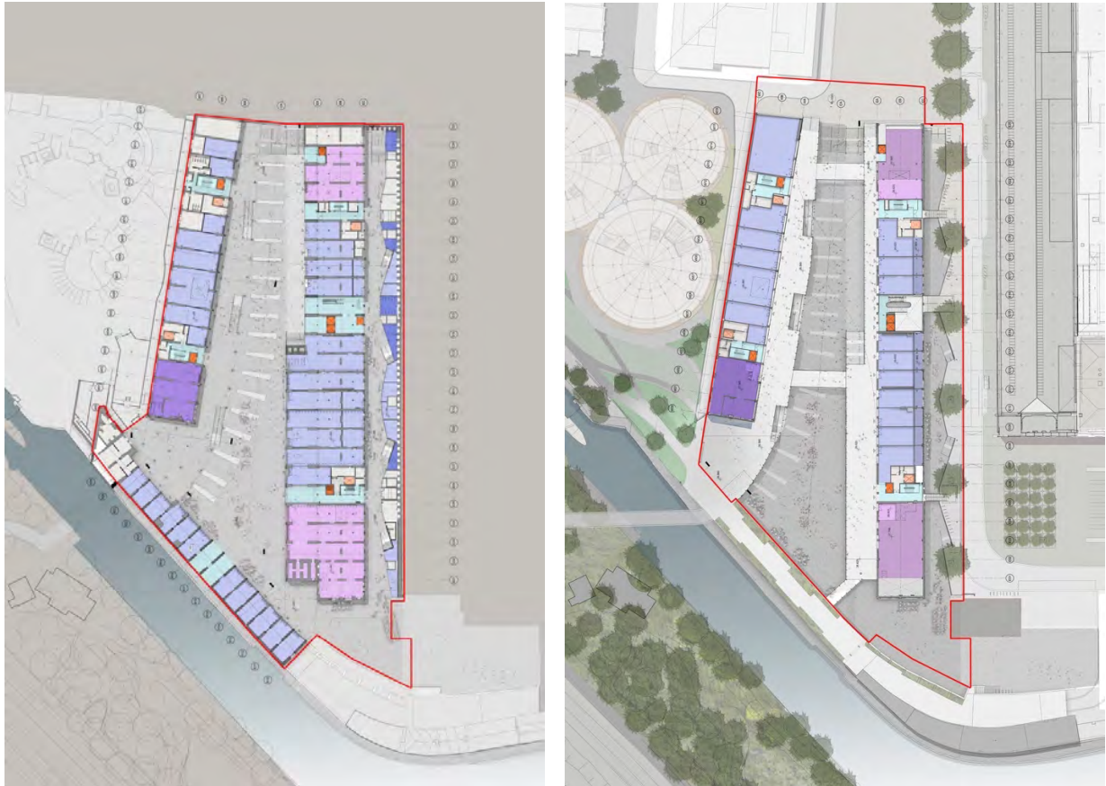
Figs 20 & 21: Plans of the Coal Drops Yard development at Yard level (left) and Viaduct level (right). The removed Plimsoll Viaduct is reflected in the yard level finish, demonstrating the importance of its removal for the north-south circulation at yard level.
