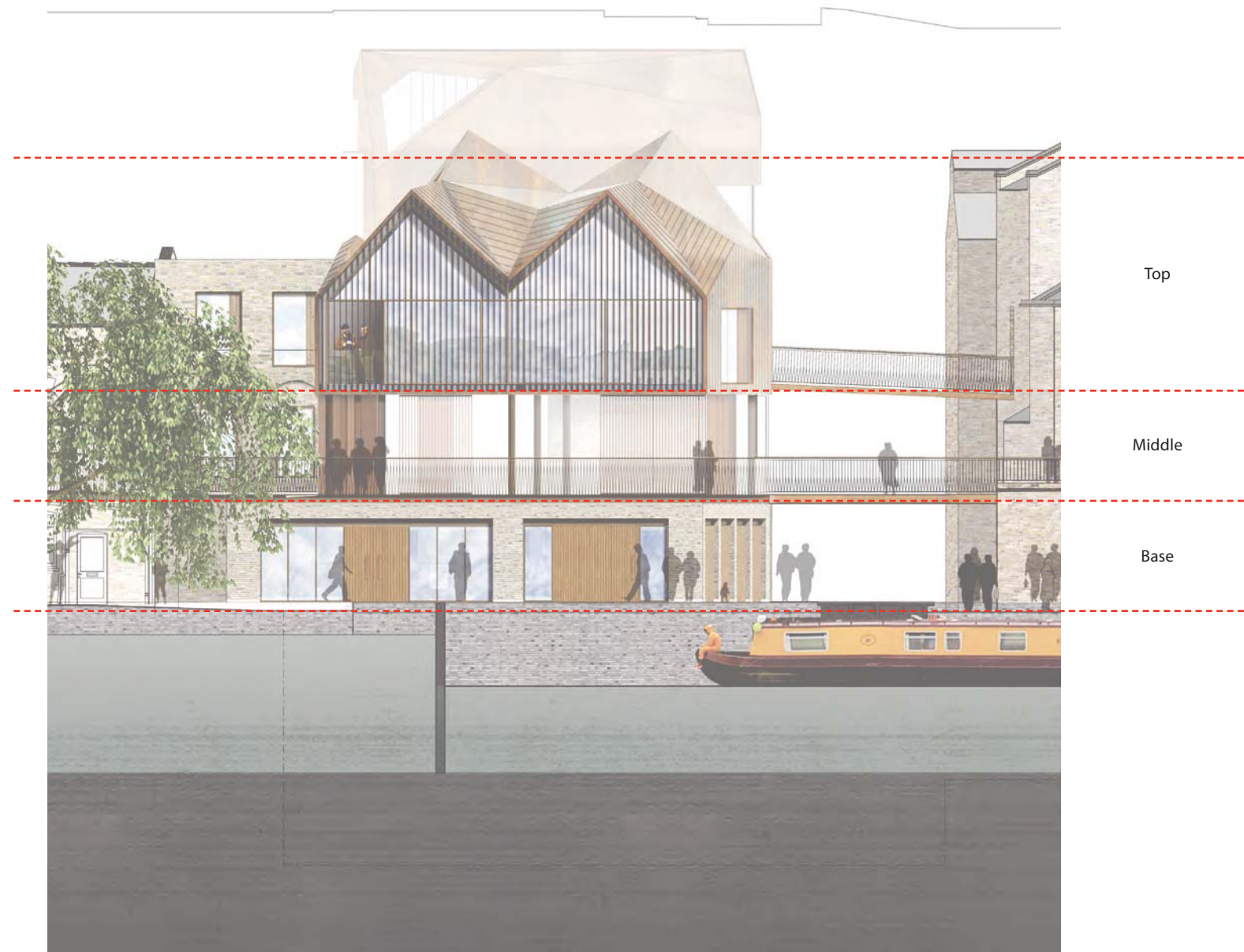
Study of canalside elevation of Middle Yard Building highlighting vertical layering
