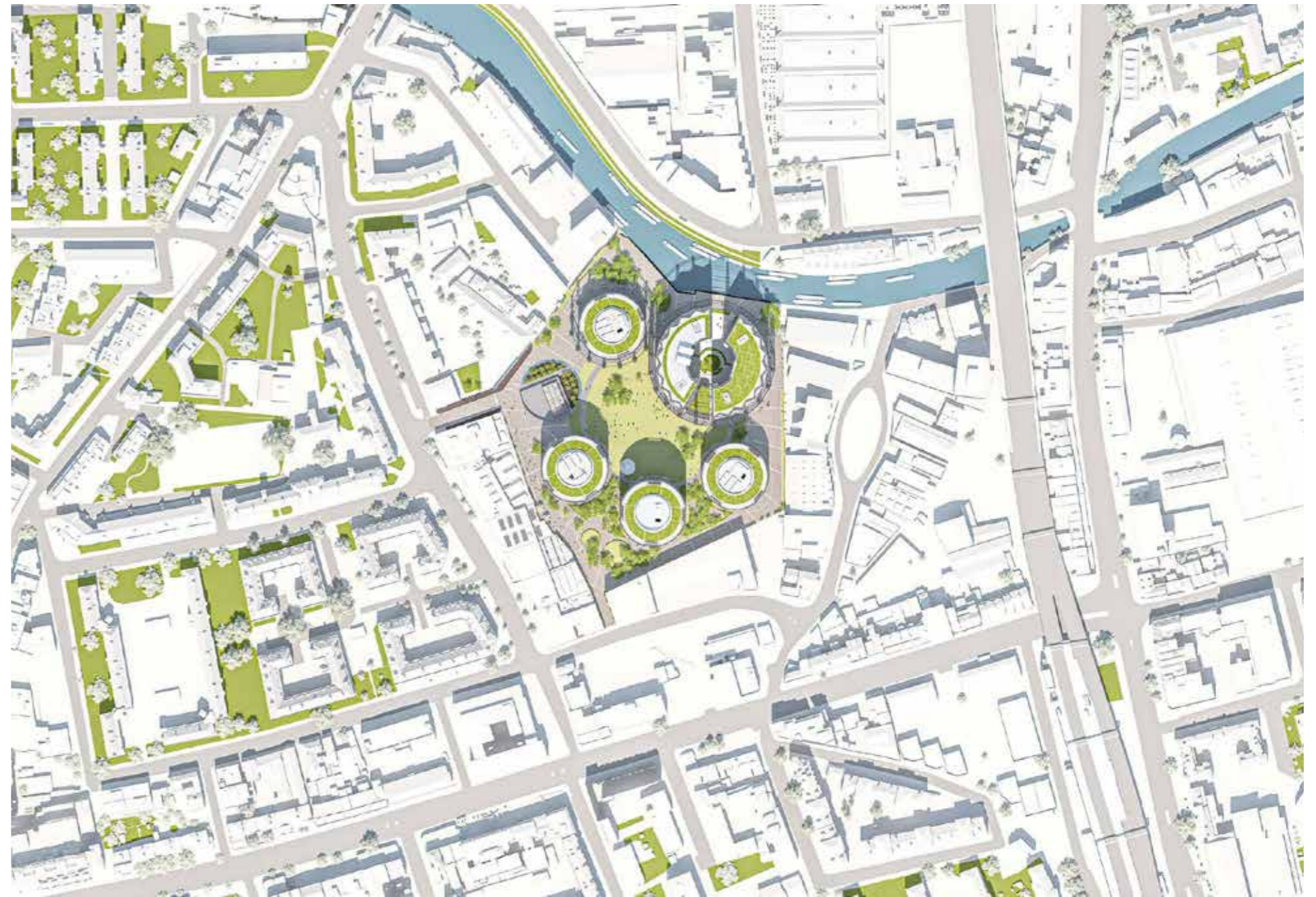
Figure 6.7 Diagram showing the layout of the circular buildings surrounding the central lawn, with shared public space along the boundaries, and in particular, adjacent to the canal.
