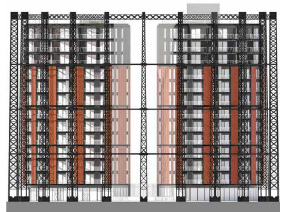
Figure 6.4 Illustration showing the general layout of the elevation treatment of Building E.
