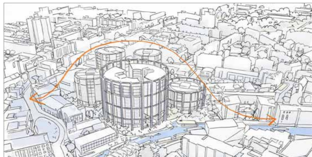
Figure 6.6 Sketch illustration showing how the scale of the development gradually steps up to the height of Gasholder No. 5, and so retaining the primacy of that structure in local views.
