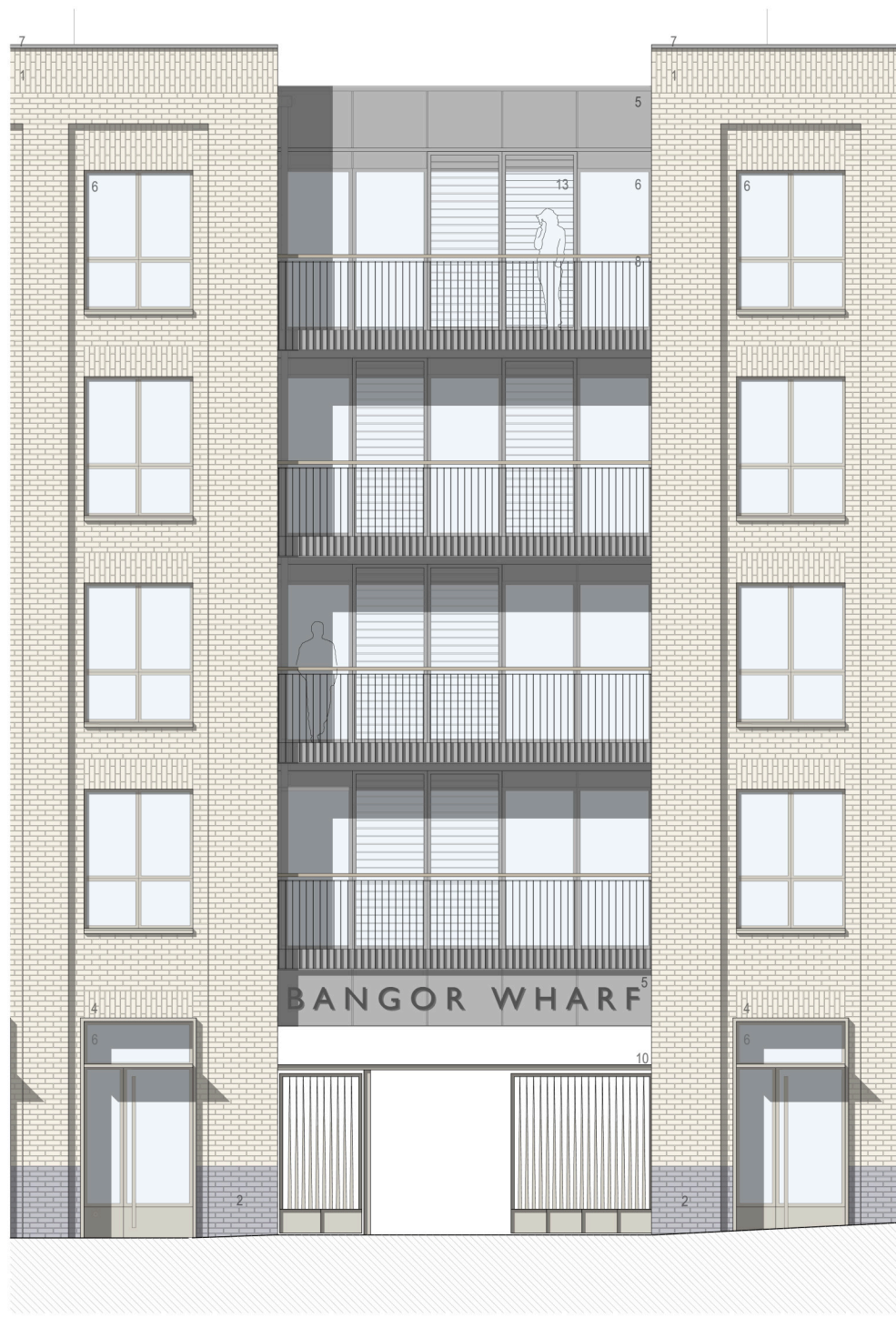
Part Elevation - Block B - Georgiana Street Scale 1:50
